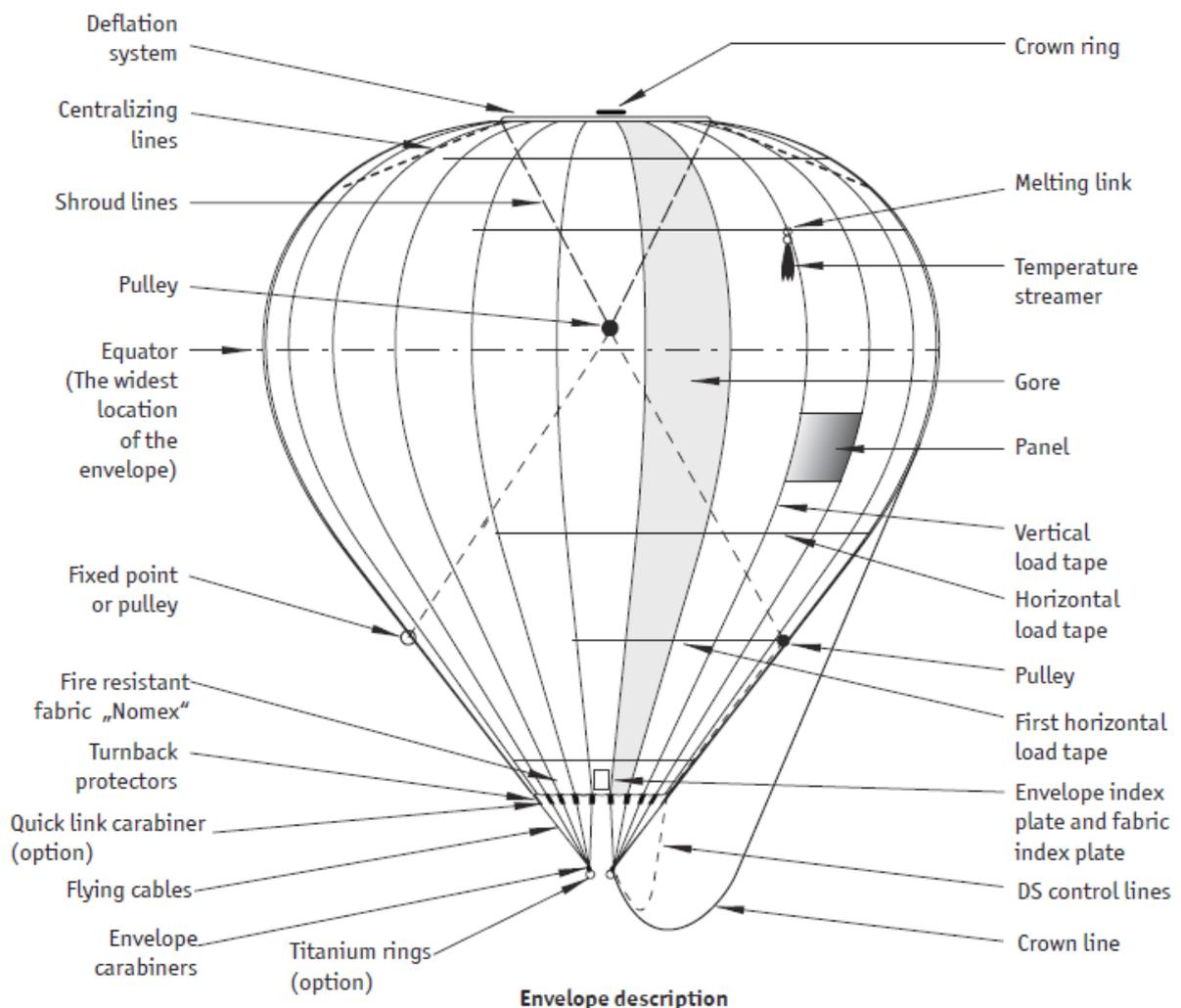
\*if titanium rings are used, they have to be fitted at all attachment points
