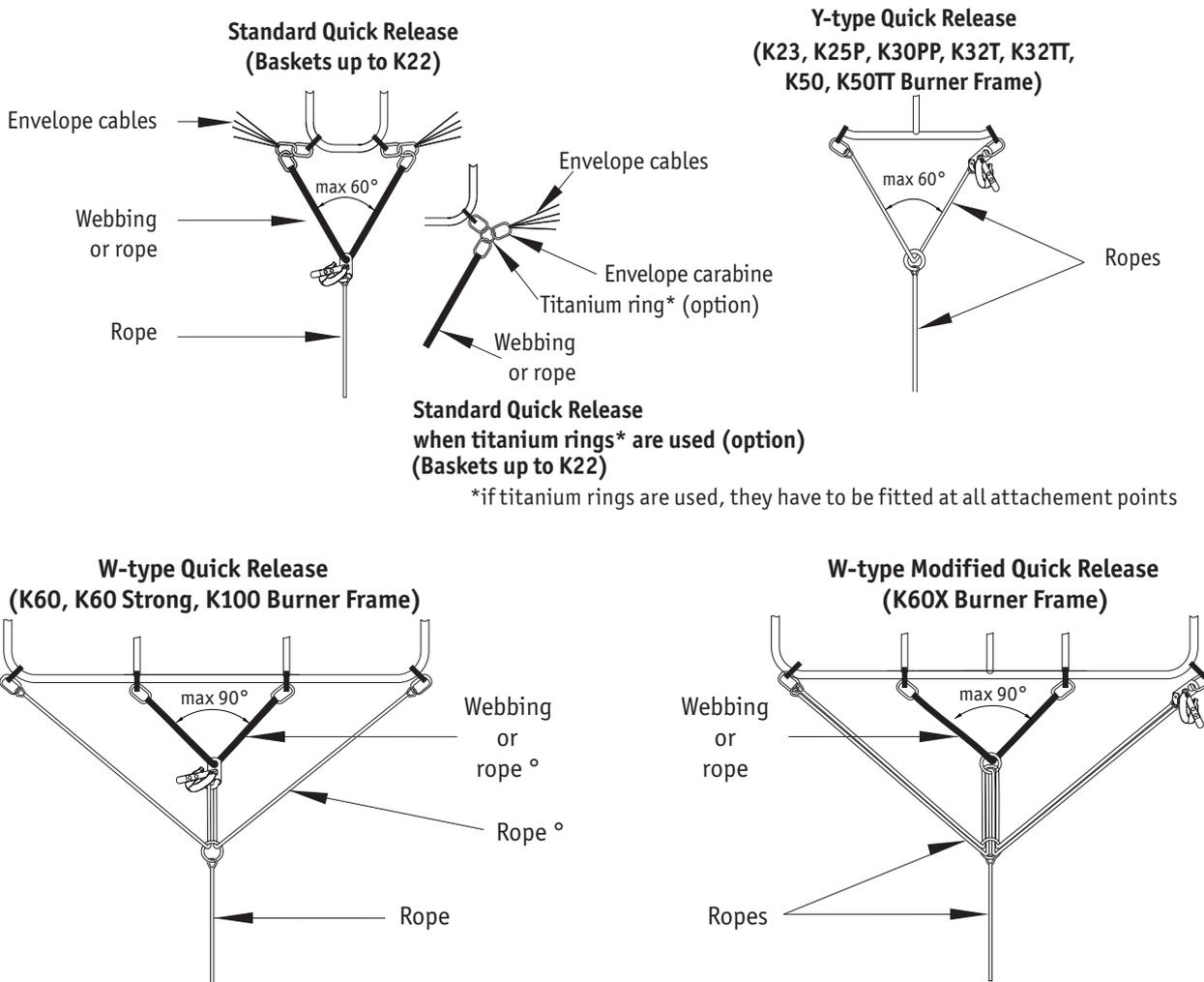
° use quick release set with red ropes when attaching to the burner frame
