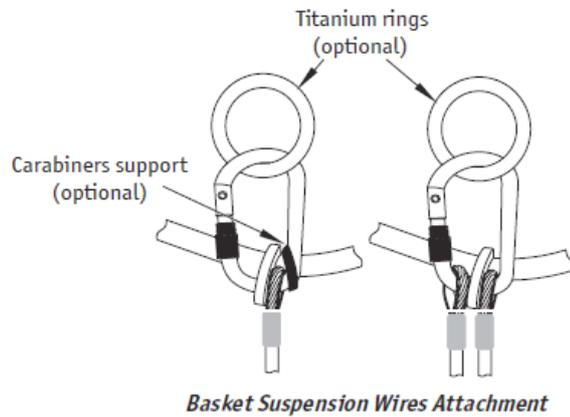
\*if titanium rings are used, they have to be fitted at all attachment points
