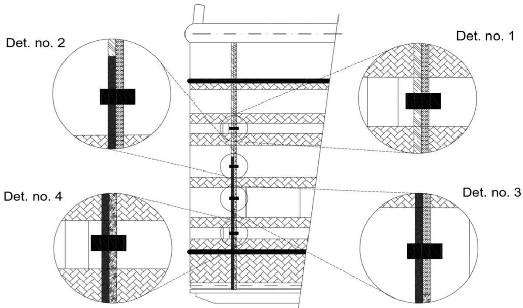
Fig. 3: Details of connection between old and new wickers
