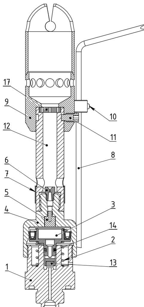
Pressure reducer and PL assembling – version of piston – separate O-ring:
