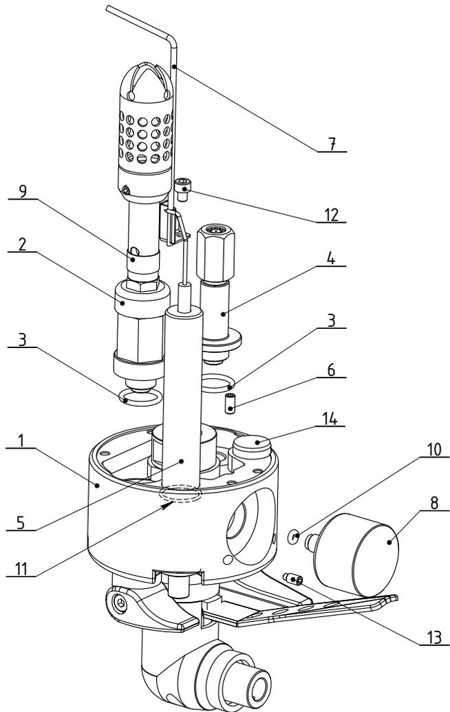
**5.1.1.2.7 Pressure Reducer (PR) and Pilot Light (PL) disassembling (B)**
