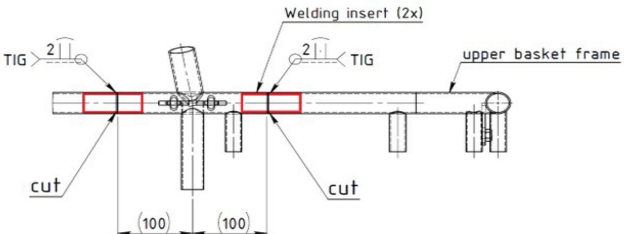
Fig. 5: Exapmle placement of cuts on upper frame basket
