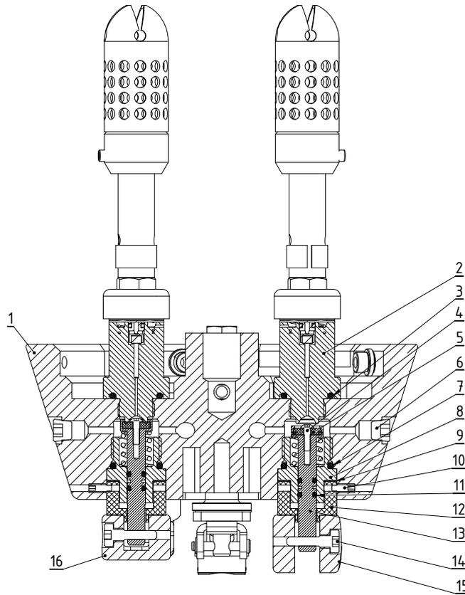
**NOTE** Socket head plug (6) don't need to be disassembled during maintenance, just in case of leaking. Plug (6) is sealed by Everseal 183 (it is possible to seal by PTFE tape alternatively).
