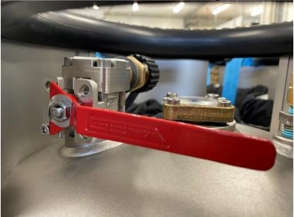
If a ball valve needs to be replaced, it is possible to replace the older type with a newer type, as the older ball valve is no longer available.
